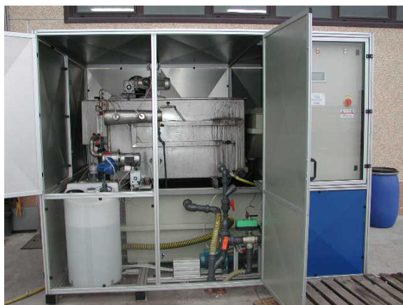
Spray box view of internal components
