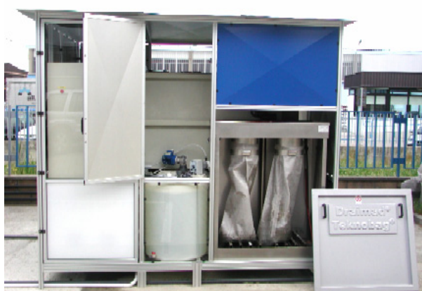
Carwash box with filtering sacks
